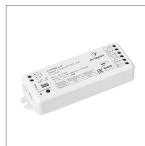
034501 | Коентроллер SMART-TUYA-WIFI-MIX-SUF (12-36V, 2x5A, 2.4G)
